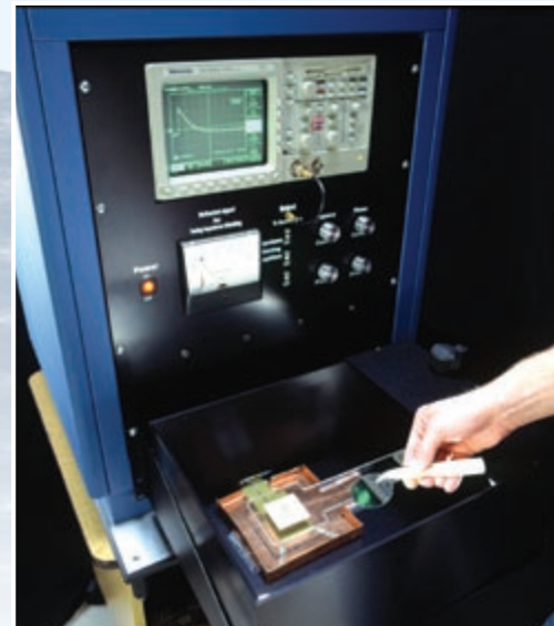
An NREL researcher loads a silicon wafer into the resonance-coupled photoconductive decay system to measure minority-carrier lifetime.
