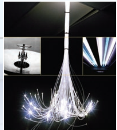
Oak Ridge National Laboratory installed a hybrid solar lighting system at Sacramento Municipal Utility District's Customer Service Center (left). Sunlight collected by such a system is routed through optical fibers to provide interior lighting (right).
