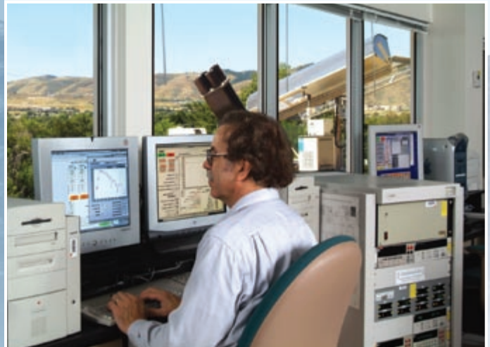
In calibrating reference cells, NREL scientists concurrently measure spectral irradiance, total irradiance, and the cell's short-circuit current under outdoor conditions.
