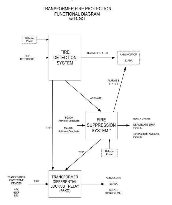
\* Includes electrical and mechanical equipment to discharge fire suppression water. Deluge type should cycle or use high level detection to limit water volume and overflow risk.
