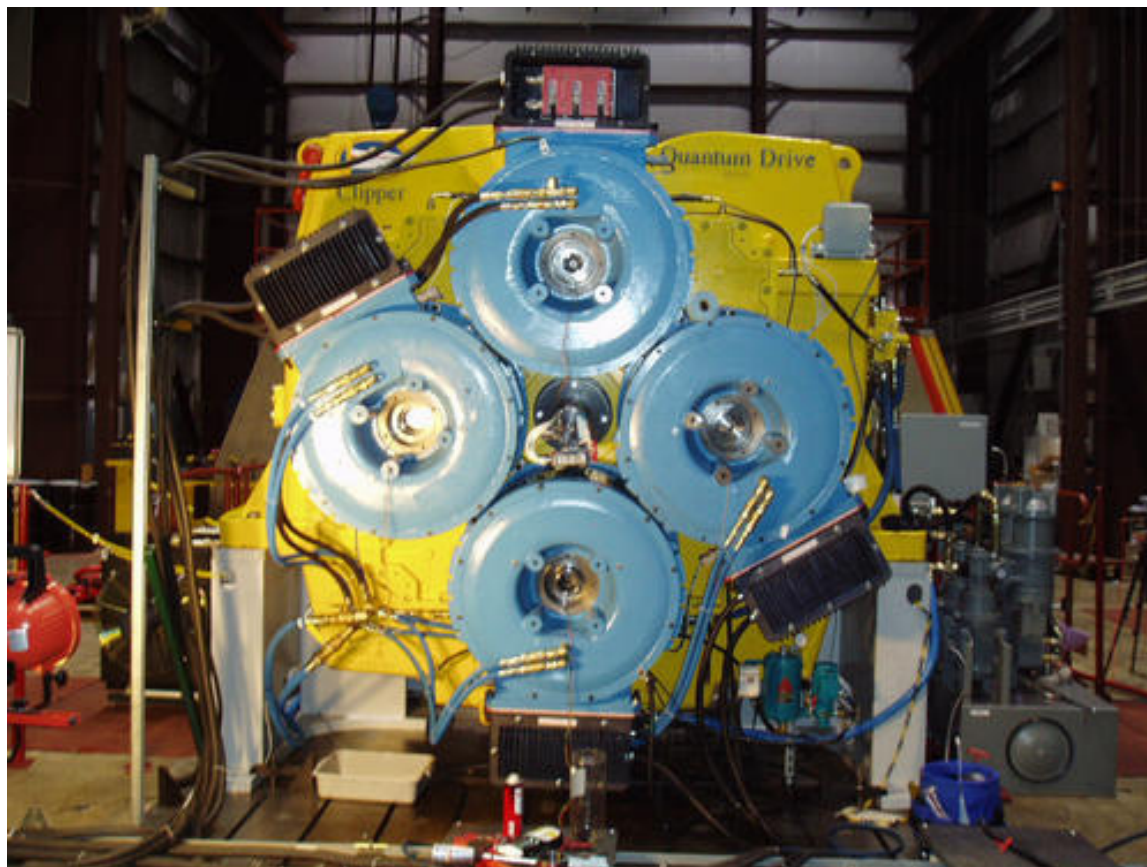
Figure 2-12. Clipper Windpower multiple-drive-path gearbox
