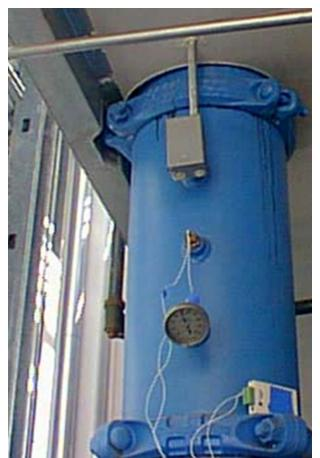
Figure 7: Water temperature sensor installed in test port ("Pete's plug") with logger; note masking tape on logger used to field note time of installation, removal time, sensor used and measurement point name.
