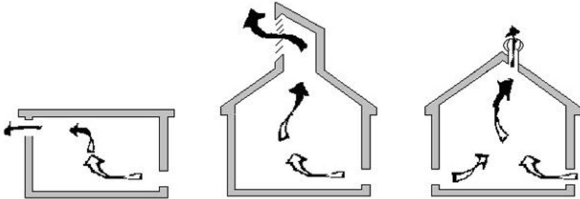
Figure 6. Air Flow Patterns Using Natural Convection
