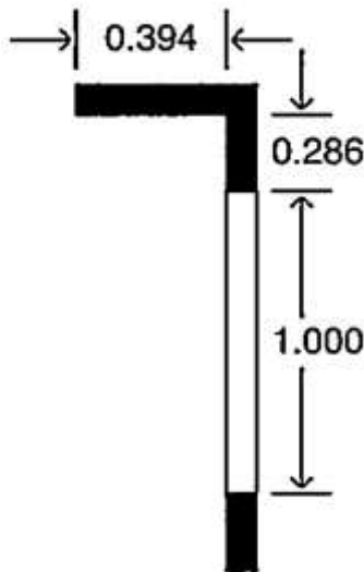
Fig. 9. Shading Geometry (not to scale) For Albuquerque, NM
