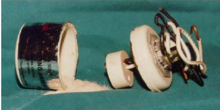
Figure 7. Unlisted Surge Protector
