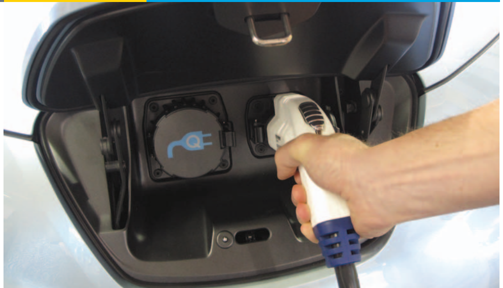
All-electric and plug-in hybrid electric vehicles are charged by plugging the vehicle into an electric power source. Photo by Andrew Hudgins, NREL/PIX 17634
