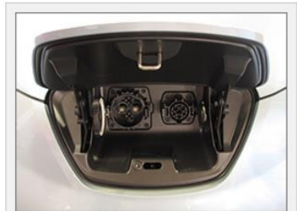
The standard J1772 receptacle (right) can receive charge from AC Level 1 or AC Level 2 equipment. The DC fast charge receptacle (left) uses a different type of connector.
