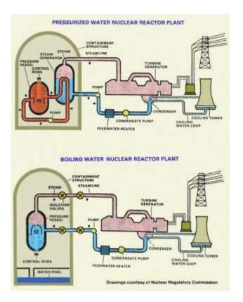
In a sense, BWRs are thought to be simpler to protect in an accident situation. The reactor can be depressurized and as long as water can be pumped into the vessel core cooling is maintained. If the water boils in the core this helps remove heat. However, a source of power is necessary to run a pump. The two sources of power by design are offsite power or the electrical gird connection and onsite power from the emergency diesel generators.
