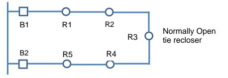
To make coordination easier, some recloser can lower their tripping characteristics when they operate in reverse mode. So, in this particular case, recloser R2 would drop its current pickup setting. Recloser R2 sees lower fault currents than it normally does and it needs to open before recloser R3 or R4. In the case fault occurs between breaker B1 and recloser R1 the loop consisting of five reclosers will respond in a similar way it would respond in the case of three-recloser loop:
