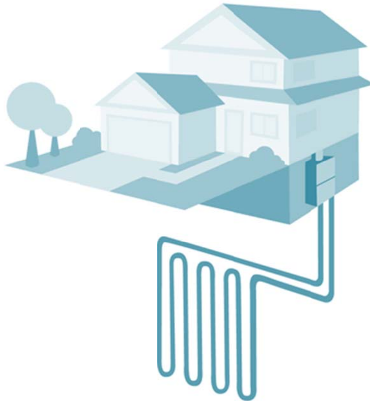
Figure 4. Vertical Ground Heat Exchanger
