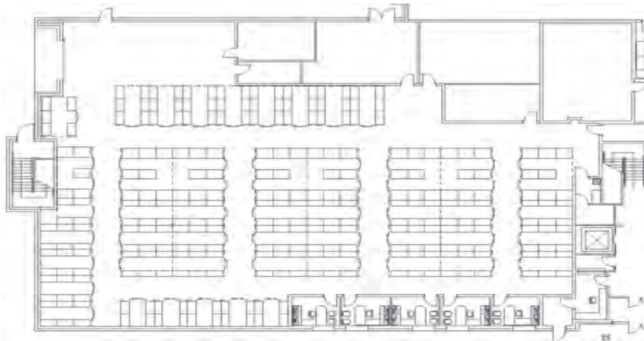
Figure 4-21 Unit Storage with Staging and Supply Office
