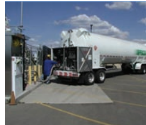
Liquid hydrogen is delivered to the California Fuel Cell Partnership hydrogen fueling station in Sacramento. Photo courtesy of CaFCP
