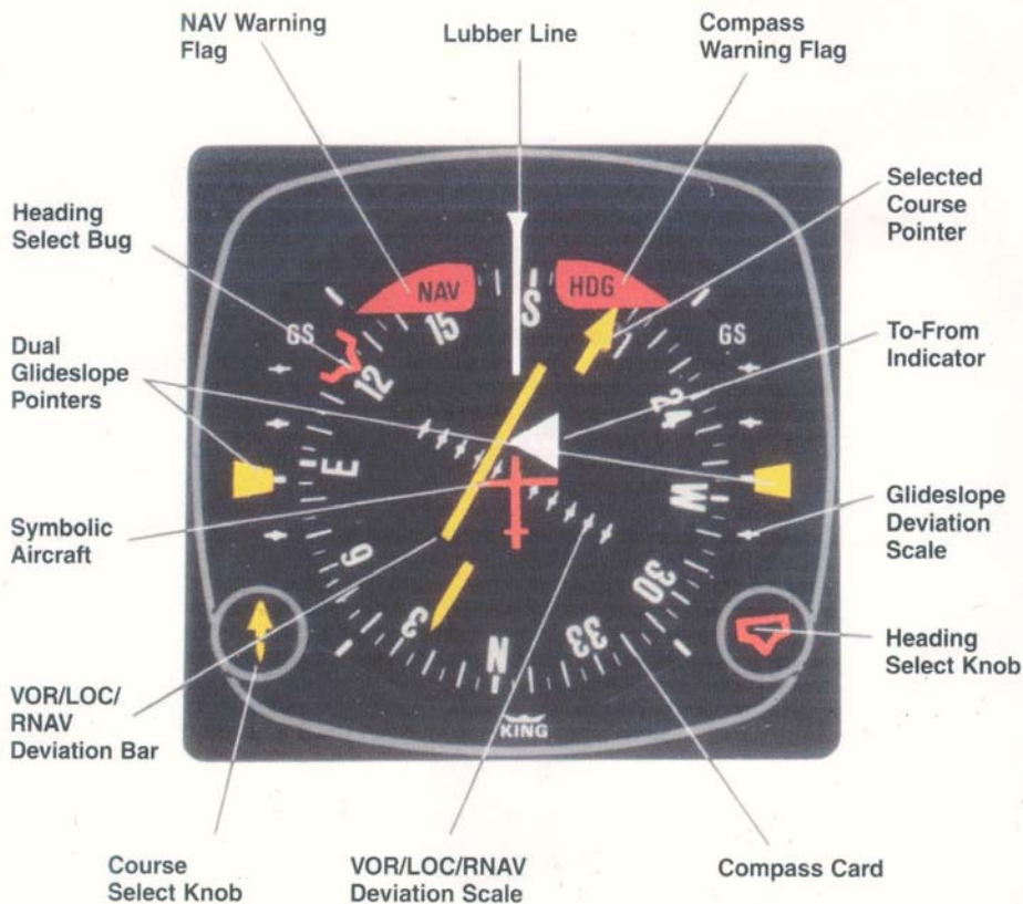
Fig D7: HSI. A Superb Advanced Instrument that Includes Several Functions. Described in great detail in later Aero Nav system in this series.
