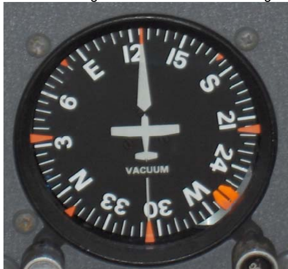
Fig D6: Vertical Card Compass; DG, Slaved Gyro, Remote Compass, or Pure Magnetic Field Powered Compass
