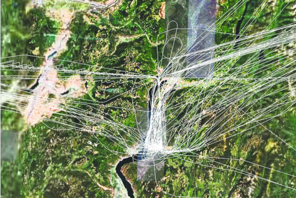
Fig 111: RNP Illustration of High Density Traffic In & Out of a Major Airport
