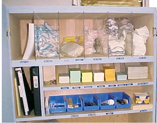
Figure 3 – Example of a cabinet after Set In Order
