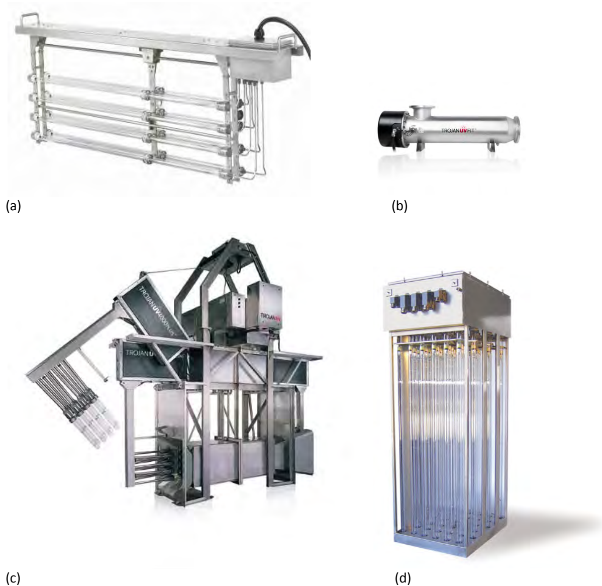
Figure 6-1. Example UV Lamp Configurations for Wastewater Treatment (a) Calgon C 3 150 for open channel flow, horizontal and parallel lamp arrangement (b) TrojanUVFit for closed channel flow (c) TrojanUV4000Plus for open channel flow, horizontal and parallel lamp arrangement, and (d) Aquaray® 3X Vertical Lamp System for open channel flow, perpendicular lamp arrangement. Used with permission.
