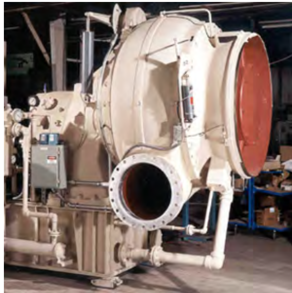
Figure 5-4. Example of Single-Stage Centrifugal Blower with Inlet Guide Vanes and Variable Diffuser Vanes by Turblex®. Used with permission.
