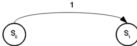
Figure 2 - a transition from state S_0 to state S_1 as a result of an input of 1
