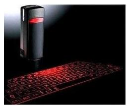
These high-tech keyboards have been around since 2003 though you have likely never heard of them. Instead of a physical keyboard, the Virtual Keyboards project the image of a keyboard onto a smooth surface. Then, depending on which beam of light gets blocked, the sensor can detect what key you are pressing. This is a wonderful gadget for an on-the-go professional who can't stand the
