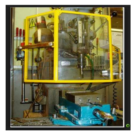
Below is given proper guarding techniques for rotating components of high-speed equipment. Please note, in the figures above and below, a specific color, yellow, is used to bring attention to the guards. This is common practice in manufacturing and should be followed to indicate the presence of guards in general.
