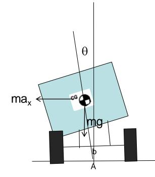
b = Distance between Suspension  $\theta$  = Angle of Sway
