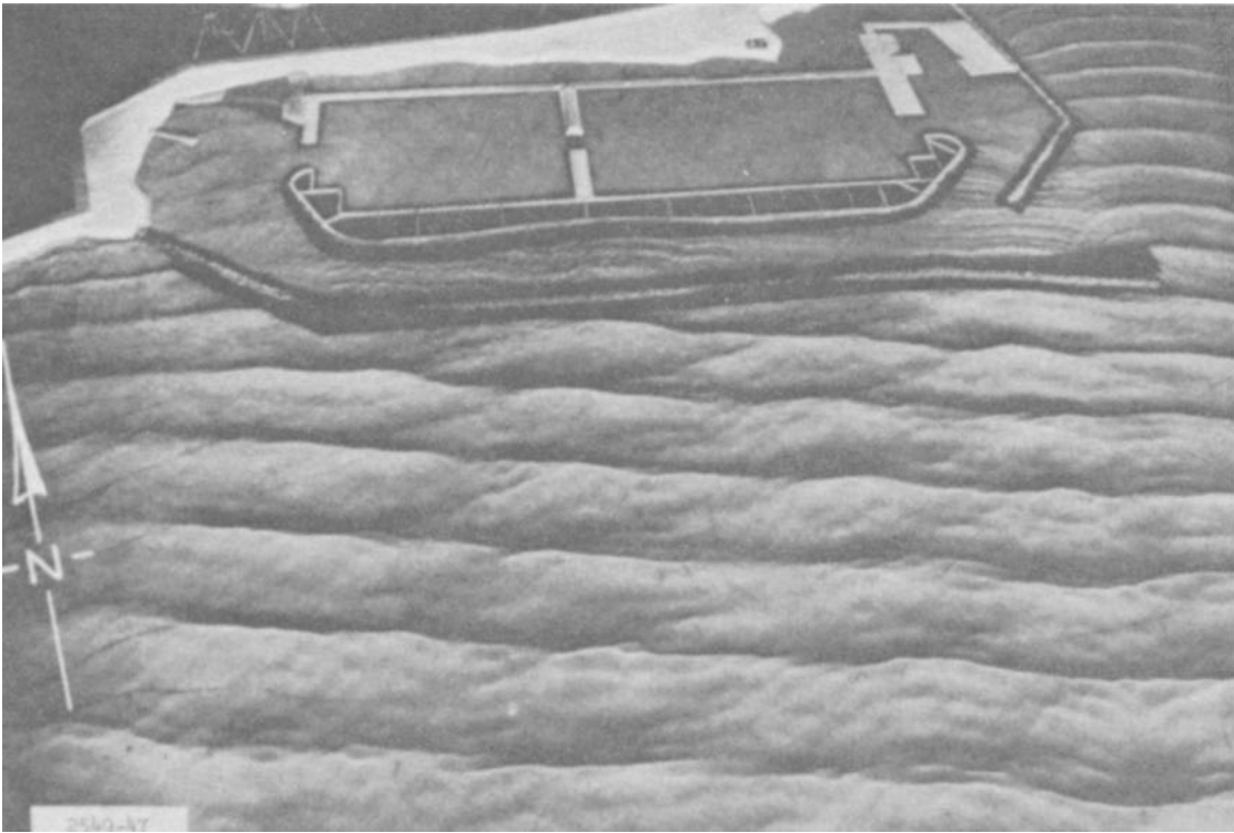
Figure A-4. Wave patterns for the recommended improvement plan, Dana Point model.
