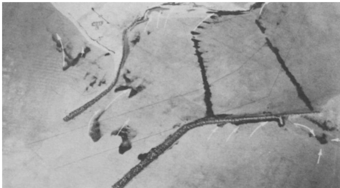
Figure A-42. Typical tracer movement for existing conditions, Newburyport Harbor.
