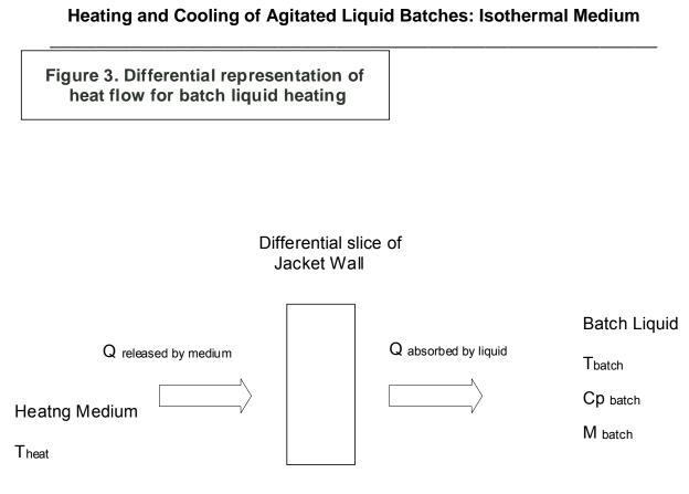
Area = A <sub>jacket</sub> Heat transfer coefficient = U <sub>jacket</sub>
