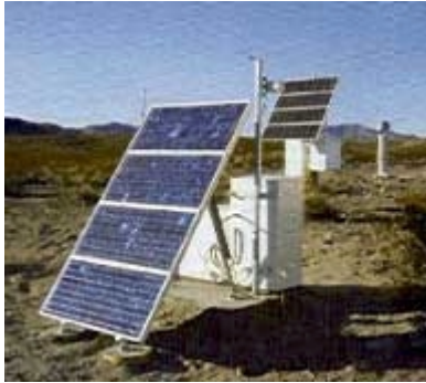
Figure 15: A prototype Earthscope station houses a GPS receiver, a seismograph, a power system and a communications link.
