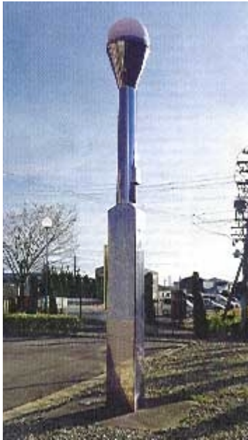
Figure 13: One of Japan's GPS receivers used for monitoring earth movements.
