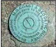
Figure 1. USGS disc set in stone.
