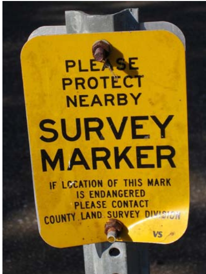
Figure 40. A county monument witness sign, Florida.
