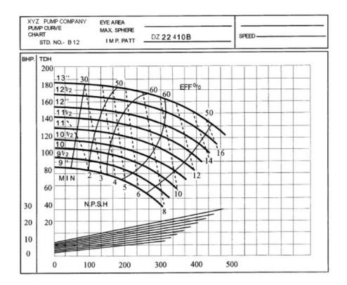
Lines of constant efficiency are plotted on manufacturer's pump performance curves as superimposed incomplete parabolic arcs generally opening in the positive direction. An rough estimate of the efficiency value using these plots is sometimes the best that can be accomplished from the pump performance curve.
