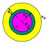
$R_1$  and  $R_2$  show the inside and outside radius of the pipe.
