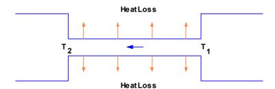
The fluid is flowing from equipment 1 at temperature  $T_1$  to equipment 2. In order to predict  $T_2$  for a given insulation thickness, we first make the following assumptions:
