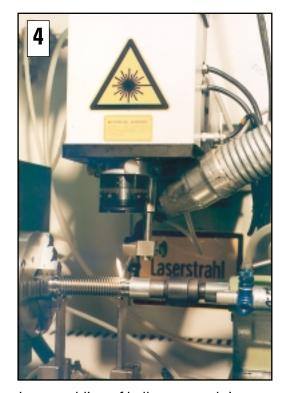
Laser welding of bellows to end rings.
