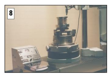
Concentricity testing of bellows, end fittings.
