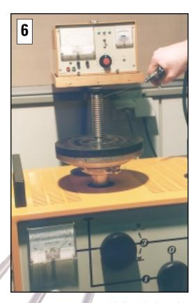
Helium leak testing. Bellows are rejected if leakage exceeds 10<sup>-8</sup> cm<sup>3</sup> per second.
