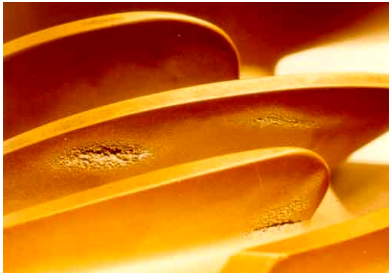
Figure 5 – Localized damage has the appearance of fatigue failure (Source: Ref. 3, Fig. 6.3) 11
