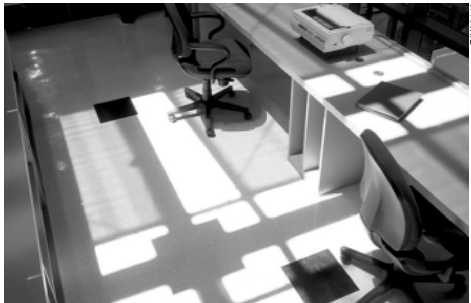
This office interior view demonstrates the quality of light transmitted by the approximately 5% translucent BIPV panel skylight.
