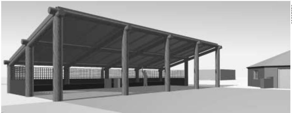
Each new BIPV structure at the Seba Dalkai School will serve as an open-air classroom supported by timber columns in a concrete foundation.
