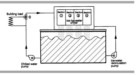
Figure 3. Typical ice-harvesting configuration. (b)
