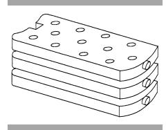
Figure 12. Eutectic salt containers. (e)
