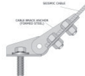
Figure 129: Cable attached with bolts to a bracket.
