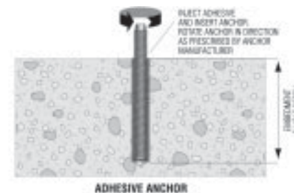
Figure 110: Adhesive anchor installation.
