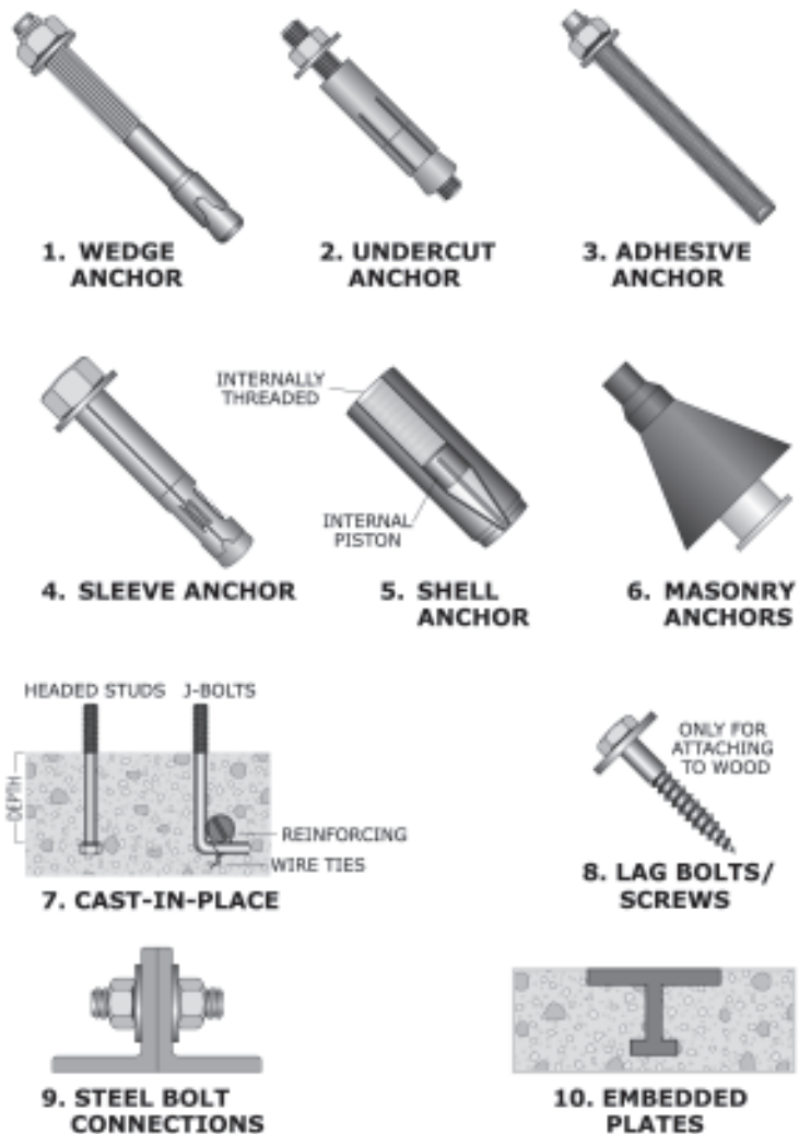
Figure 130: Types of anchors.
