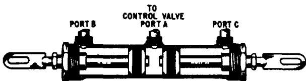
Figure 10-7.—Three-port, double-acting actuating cylinder.
