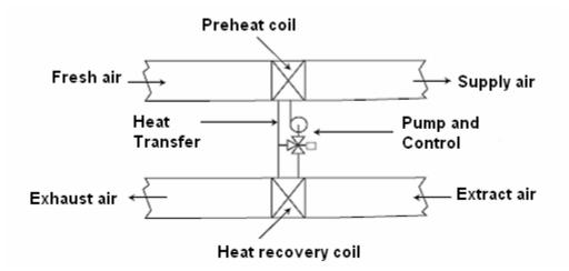
The coil in the exhaust air and the coil in the fresh air are linked with a closed water (or water-glycol mixture if frost is expected) circuit and a circulation pump. The heat is first transmitted from the exhaust coil to the water circuit and then to the fresh air coil via the second coil. The thermal efficacy is usually 45% to 55%.
