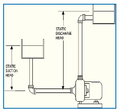
**NPSHa** = Static head + Atmospheric pressure (converted to head) + Vapor pressure of the fluid (converted to head) – Friction loss (in the piping, valves and fittings);
