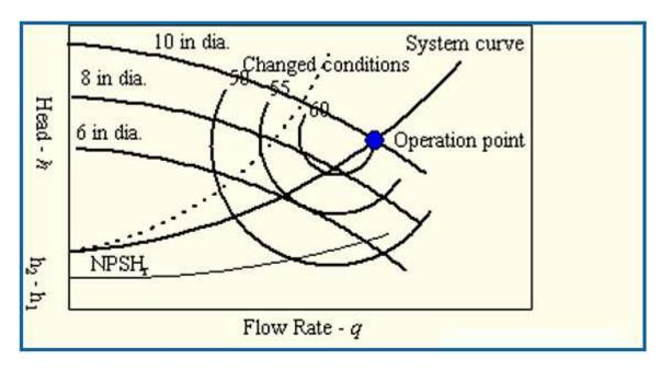
**Note**: The available NPSH<sub>a</sub> of the system should always exceed the required NPSH<sub>r</sub> of the pump to avoid vaporization and cavitation of the impellers and pump inner walls. The NPSH<sub>a</sub> is also calculated to avoid that head loss in the suction pipe and in the pump casing, local velocity accelerations and pressure decreases, start boiling the fluid on the impeller surface.
