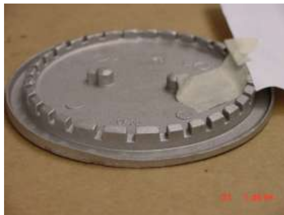
Figure 14—Burner Cap with Burner Ports and Positioning Pins
