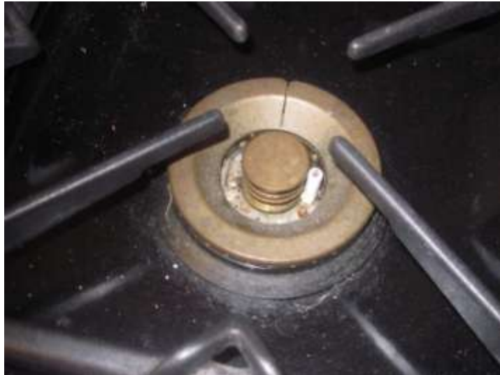
Figure 10—Position of Spark Igniter
