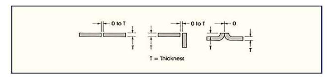
A **backing strip** is sometimes used on the opposite side of a square-groove weld. The **backing strip** keeps the molten weld metal from falling through and permits the use of more heat which results in better fusion. The welder can make a strong square-groove weld that completely penetrates the joint.
