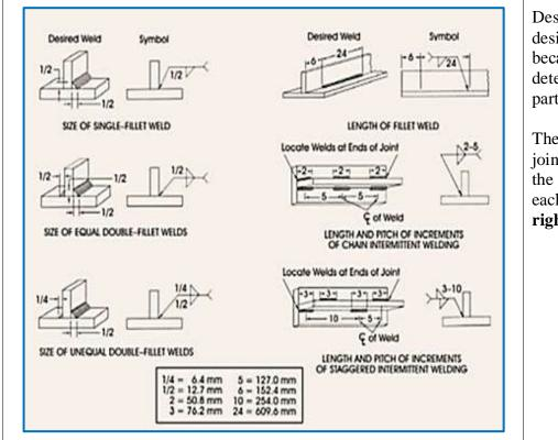
Designers need to specify the desired sizes of fillet welds because welders usually can't determine the dimensions of the parts to be welded.
