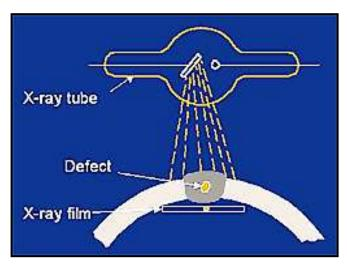
Radiographic inspection is a nondestructive inspection technique which involves **taking a picture** of the internal condition of a material. This picture is produced by **directing a beam of short wave-length radiation (X-rays or gamma rays)** through a material that would be opaque to ordinary light.
