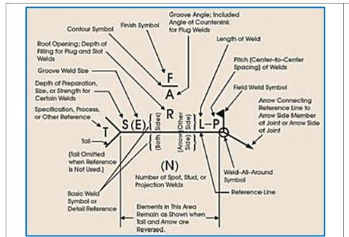
The basic and supplementary symbols are combined with other elements to produce the complete welding symbol as shown aside.
