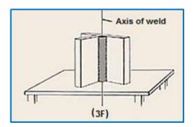
**Note:** Welders should be tested according to a qualified Weld Procedure Specification (WPS). However, welding vertically in a downward progression does not fit within the guidelines of AWS D1.1-2010, Clause/Sub-section 3.7.1).
