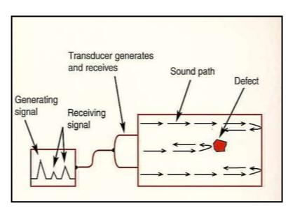
The ultrasonic vibrations are converted to electric signals, amplified, and **displayed on a Cathode Ray Tube (CRT)** screen. Because of the high frequency (above the range for the human ear), the short wavelength **allows small flaws** to be detected.
