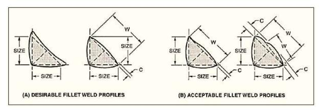
**Note**: Convexity, C, of a weld or individual surface bead with dimension W shall not exceed the value of the following table.
