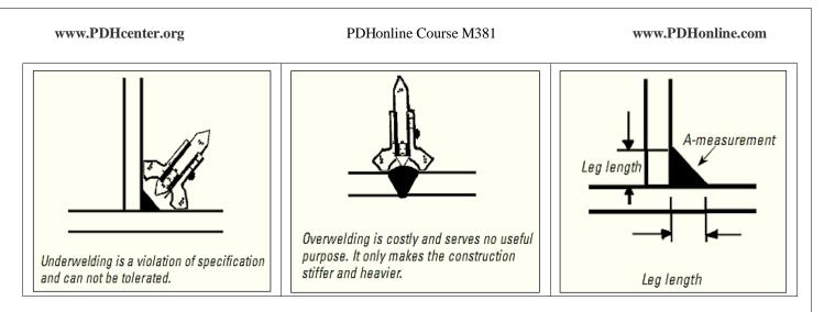
**NOTE:** For **supplemental information** and **safe welding procedures** consult the American Welding Society (AWS) *Welding Handbook* and AWS D 1.1. Joint design practices for vessels see Section VIII of the ASME Boiler and Pressure Vessel Code, ANSI B31.1 for piping and the AISC (American Institute of Steel Construction) for steel construction.
