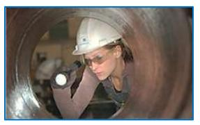
Welds must be cleaned from slag to make inspection for surface flaws possible. A **10x magnifying glass** is helpful in detecting fine cracks and other faults. As indicated before, a **borescope and dental mirrors** are useful for inspection inside vessels, pipe, or confined areas.
