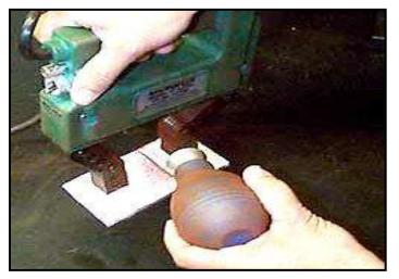
The procedure conforms to **ASTM E 138, ASTM E 709, MIL-I-6868** and the ASME Boiler and Pressure Vessel Code, Section V.
