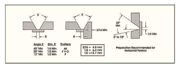
7) V-groove Weld Penetration:
