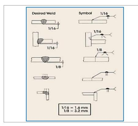
Weld penetration beyond the depth of the groove is indicated aside. The first dimension gives the depth of penetration into the groove; the second dimension gives the additional penetration into the joint root.
