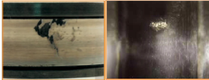
Spalling from debris or raised metal
