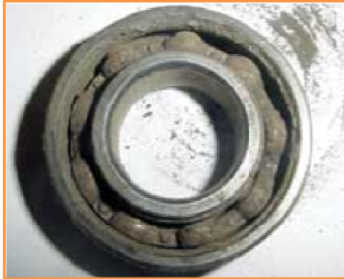
Gross contamination resulting from harsh operating conditions and/or seal failure
