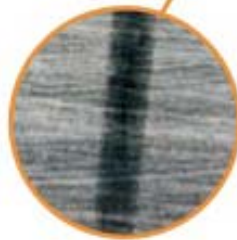
Damage from shock or impact
