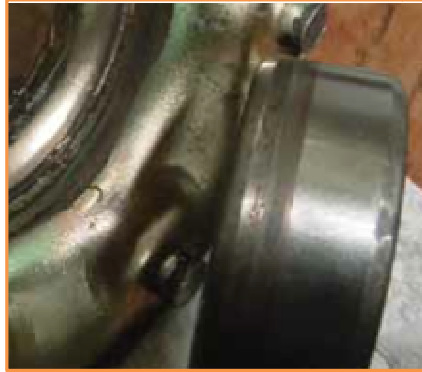
Bearing supported by only one-third of its outer ring width within housing
