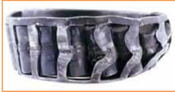
Total bearing lock-up due to skewed rollers
