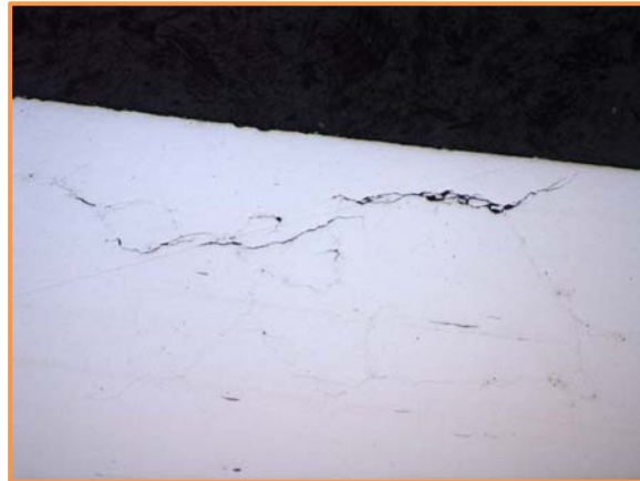
Cross section showing subsurface cracking
