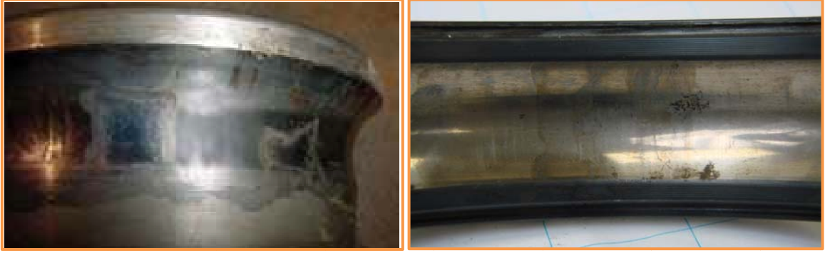
Chemical reaction of grease and moisture in a prolonged static condition resulting in pitting and corrosion as evidenced by witness marks generated at each ball location on the inner race
