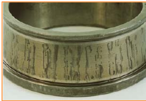
Rusting with pitting: corrosion from moisture/water exposure
