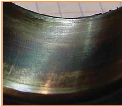
Loose inner ring fit on a rotating shaft resulting in discoloration from heat generation
