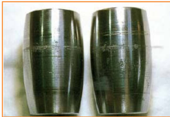
Abrasive wear due to fine particle contamination
