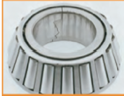
Cone bore fracture due to out-of-round or oversized shaft
