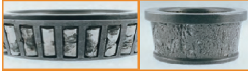
Rapid and deep spalling caused by unusually high stresses (left) and fullrace widthfatigue spalling caused by heavy loads (right)
