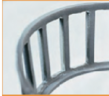
Cage pocket wear due to heavy contact between the rollers and cage pocket surfaces caused by bearing operating too loosely
