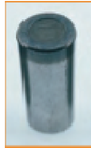
Inadequate lube film results in localized high temperatures and scoring at the large ends of the rollers
