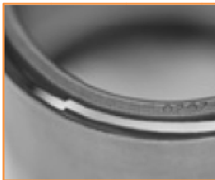
Lip damage caused by improper installation
