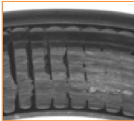
Damage on locked rollers
