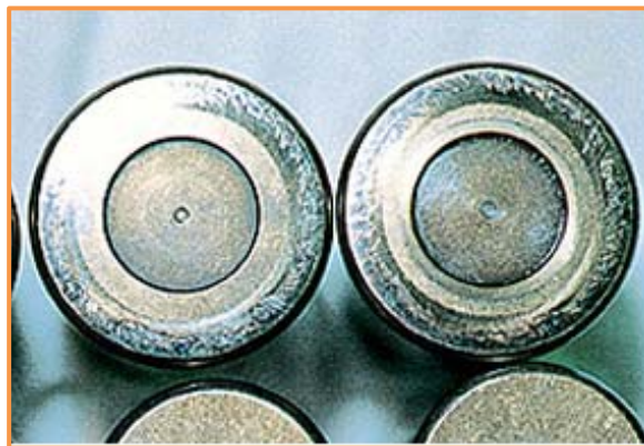
Roller end scoring due to metal-to-metal contact from breakdown of lubricant film
