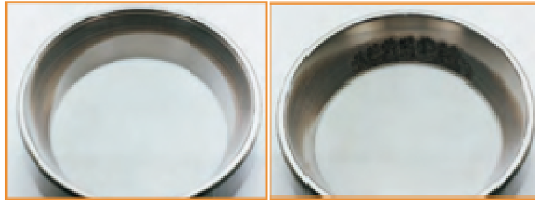
Irregular roller path from misalignment
