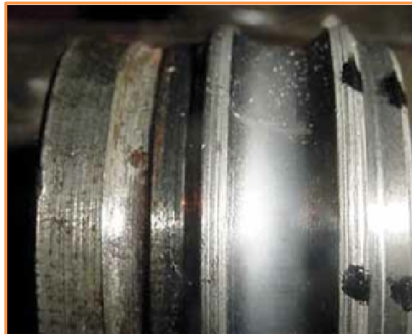
Fine particle abrasive wear on inner race, commonly known as frosting
