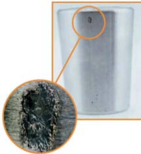
Electric arc pitting: small burns created by arcs from improper electric grounding while the bearing is stationary
