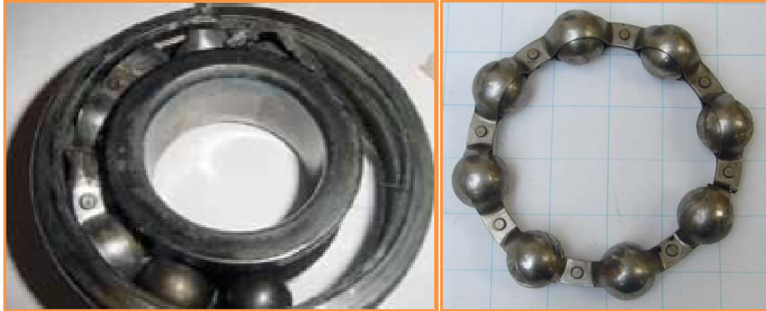
Cage damage due to misalignment or excessive speed
