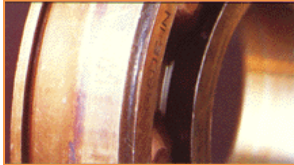
Heat discoloration on race
