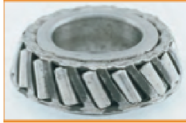
Rollers binding and skewing due to the cage ring being compressed during installation or interference during service
