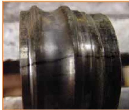
Axial crack on inner ring due to over-sized or out-of-round shaft
