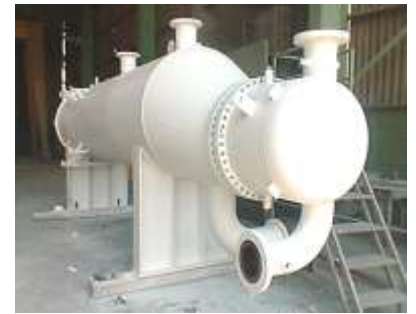
Heat Exchanger Final Painting Evaluation
