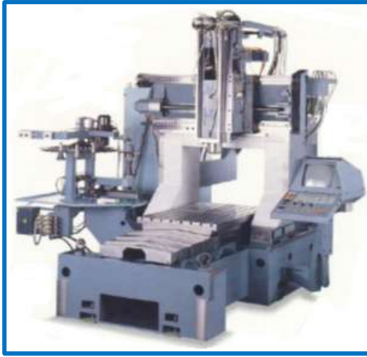
A gantry type CNC machining center
