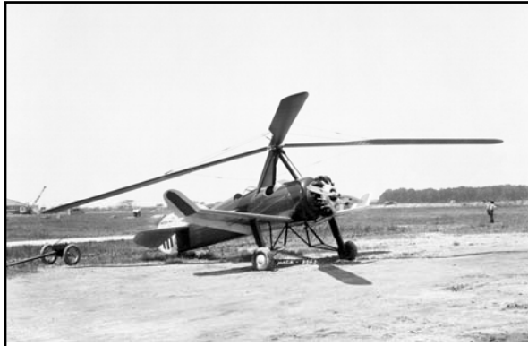
Above: caption: "Pitcairn PCA-2 Autogiro purchased in 1931 and used for experimentation. Owned and operated at Langley Field, Virginia by the N.A.C.A." 235
