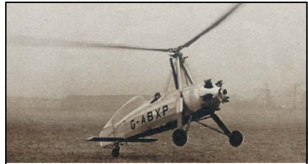
Above: caption: “An aeroplane without wings, elevators, or ailerons – the ‘direct control’ autogiro. Mr. de la Cierva landing with the tail wheel of his machine touching ground first – the rest of the aircraft then sinking slowly to earth.” 200
