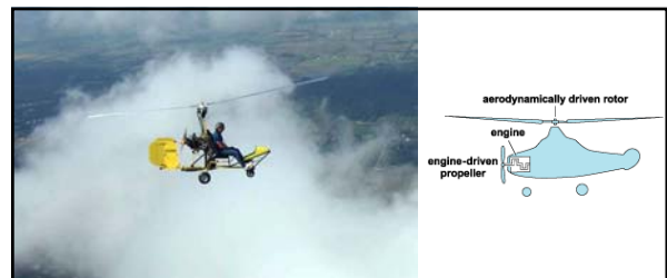
Above: Bensen Aircraft B8MG Gyrocopter. Modern Autogiros typically follow one of two basic configurations. The most common design is the pusher configuration, where the engine and propeller are located behind the pilot and rotor mast, such as in the Bensen "Gyrocopter" developed by Igor Bensen in the post-WWII era. Less common today is the tractor configuration. In this version, the engine and propeller are located at the front of the aircraft, ahead of the pilot and rotor mast (right). This was the primary configuration in early Autogiros, but became less common after the advent of the helicopter. It has enjoyed a revival since the mid-1970s. 570
