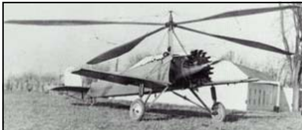
The most powerful of the six C.8s constructed was the two-seat C.8W (above) fitted with a 220-hp Wright Whirlwind J-5. Cierva had equipped the aircraft with an American engine at the request of its buyer, Harold Pitcairn (this was the Autogiro Pitcairn donated to the Smithsonian Institution). European engines turned counter-clockwise (when viewed from the rear) while the American Wright Whirlwind J-5 turned clockwise, which caused Pitcairn some apprehension over its effects on rotor rpm. After Cierva confirmed that this would not be an issue, Pitcairn agreed to purchase a new C.8 with the Wright engine. On December 11 th 1928, the C.8W arrived in the United States onboard the S.S. Aquitania . Pitcairn planned to have the Autogiro make its flight on the twenty-fifth anniversary of the Wright Brother's first powered flight (December 17 th 1903) at his Bryn Athyn, Pennsylvania airfield. However, he was conservative when dealing with the experimental testing of the newly reassembled aircraft and was extremely anxious that all should go well on the first flight. Thus, not until December 18 th 1928 would the C.8W perform the first flight of an Autogiro in the United States, with Cierva test pilot Arthur Rawson at the controls. Pitcairn flew the aircraft the following day.
