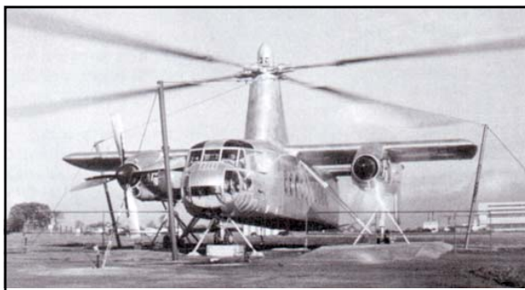
Above: caption: "Powerplant and rotor-drive testing before the first flight of the Rotodyne, in November 1957, involved some 50 hours of rotor and 100 hours of engine running" 521
