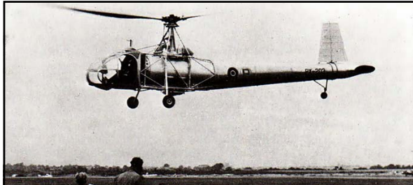
In 1945, Cierva Aircraft Company was absorbed into G&J Weir and the resulting company was called Weir-Cierva. At that time, the only helicopter under development by Weir was the W.9 (above). It was an experimental tandem design begun in 1944. Power was provided by a de Havilland Gipsy Six Series II engine with one main rotor and instead of an anti-torque tail rotor, it used a system of thrust reaction expelling air through an opening. Only one W.9 was ever built. Above: caption: "The Cierva W.9 used the push of a reactor to cancel torque reaction of the rotor" 379
