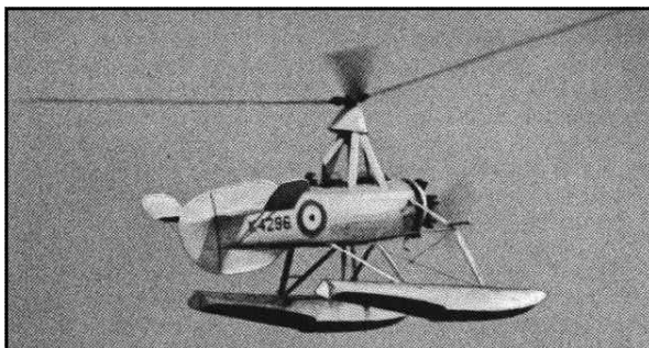
One twin-float Cierva C.30A (above) designated "Sea Rota" and ten standard Rotas (with wheeled undercarriages) were completed to Specification 16/35 (1935) 371
