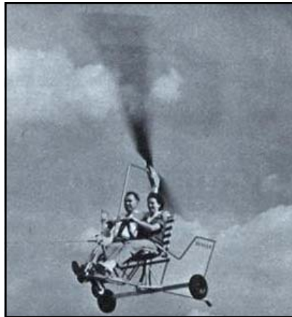
"New Model two-seat Gyro-Glider has no engine. It soars when towed by a car or motorboat and is controlled in the air by an overhead stick, like a full-size helicopter. The craft weighs 98 pounds and totes a 500-pound pay load. It takes off at 25 mph and cruises at 35 mph. In a strong wind it can be flown like a kite on a long rope tied to the ground. Kit ($100) and plans ($10) are available from Bensen Aircraft Corp., P. O. Box 2746, Raleigh, N. C. Solo in three hours!" Mechanix Illustrated, Nov. 1959 567
