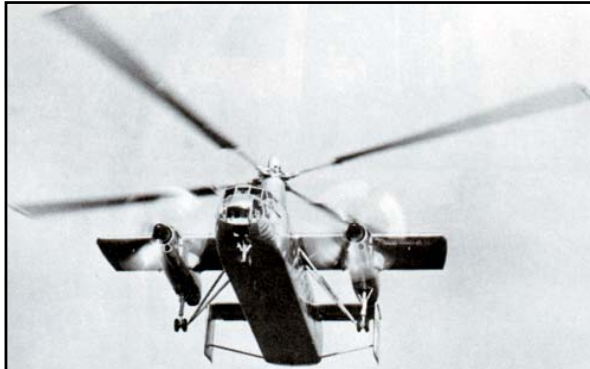
Above: caption: "This picture of the Rotodyne, on one of its first flights, shows the massively strutted fixed undercarriage which, pending redesign, replaced the retractable gear for the early tests" 517
