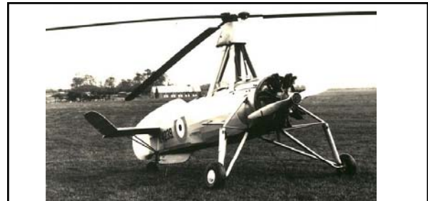
The prototype C.30 (above) differed chiefly in having a tripod rotor pylon and dihedral on the tail plane tips; the fuselage was modified from a standard Cierva C.19. The first customer for the production C.30A was the Royal Air Force for whom the type was built by Avro and given the name “Rota.” During 1933, the C.30 prototype was converted for jump-start trials with a modified rotor head (in 1936 another prototype made the first genuine vertical take-off by an Autogyro by keeping the engine and rotor system engaged throughout the take-off sequence). This machine was, in effect, the prototype for the C.40, five of which were ordered for the RAF as the Rota II. These were built by the British Aircraft Manufacturing Co., having side-by-side seats, a wooden semi-monocoque fuselages and a 175-hp Salmson 9NG engine. 364
