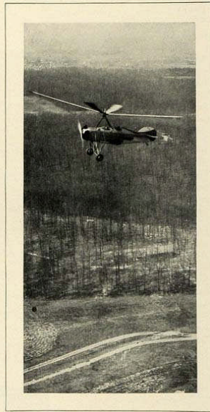
COMPARATIVE AREA REQUIRED FOR SAFE LANDING OF AUTOGIRO AND AIRPLANE—COMPARATIVE DATA 300 H. P. PITCAIRN AUTOGIRO—300 H. P. PITCAIRN MAILWING
