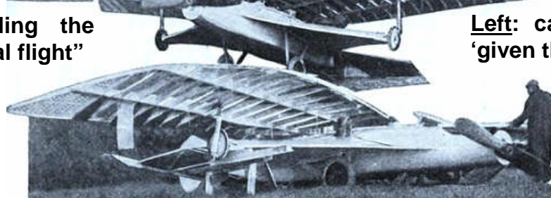
Above: caption: “Shown above is all that was left of the novel bird-plane after it had shaken itself to pieces. The inventor expects to rebuild it, using stronger metal throughout to strengthen the construction”
