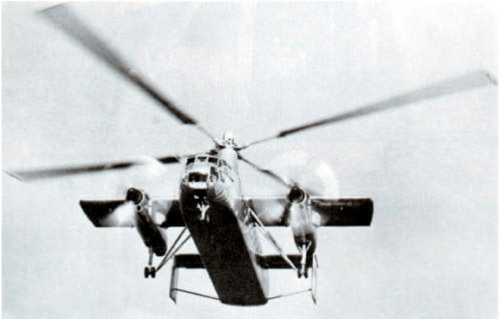
Above: caption: “This picture of the Rotodyne, on one of its first flights, shows the massively struted fixed undercarriage which, pending redesign, replaced the retractable gear for the early tests”
