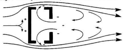
Flow through a building with all windows on leeward or sidewalls (poor ventilation as all windows are in suction)
