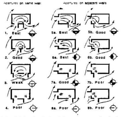
A. Wing wall design patterns for two windows on the same or adjacent walls snowing probable airflow patterns and wind directions for improved ventilation performance due to wing walls.
