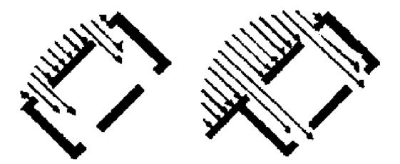
Wingwalls can increase the elevational area of the building and increase the positive pressure build up and interior velocity. The lengths of the arrows suggest the relative pressure differences.
