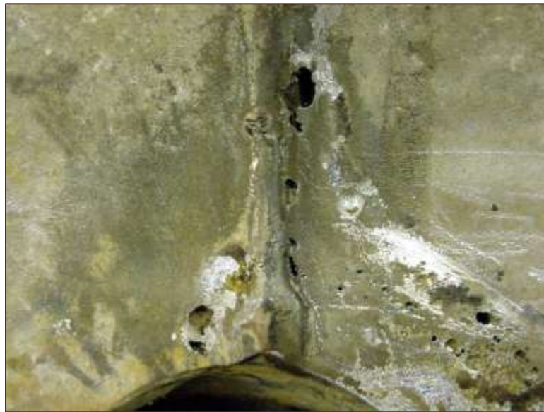
MIC attack in weld zones of a stainless steel component
