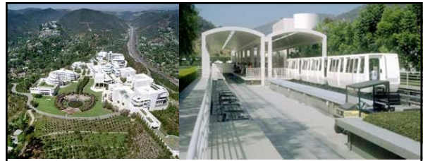
Above L&R: a windswept hilltop in California's Santa Monica Mountains is home to the J. Paul Getty Center , one of the world's largest private museums. Each year, thousands of people visit the center, transported from a parking area below by the Otis Hovair system; a state-of-the-art people-mover system installed in 1998. The Otis system uses pollution-free, noiseless electronic motors to propel two shuttle trains on a cushion of air along a curved line that follows the hillside's jagged contours up a 209-foot vertical rise.
