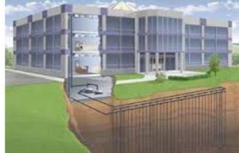
Figure 10 Deep Vertical Wells for Large Commercial structure
