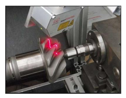
FIGURE 25: COUNTING TEETH ON A MILLING TOOL
